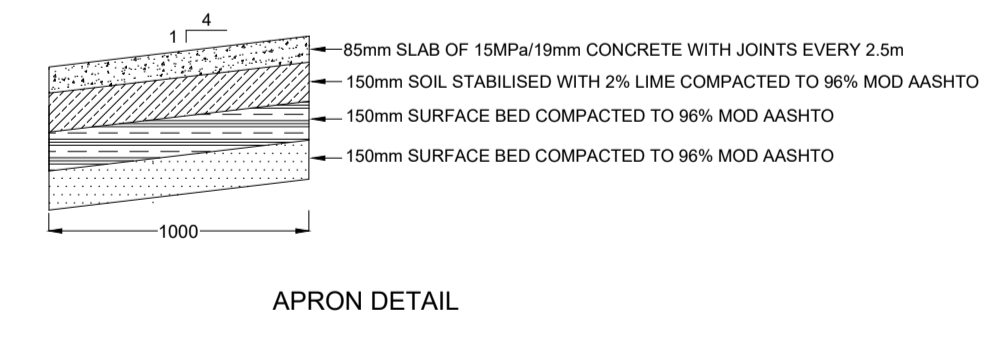
FOUNDATION DETAILS - SECTIONS
